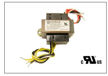
The Ingram UL Class 2 Transformer is a multi-tapped primary, dual winding secondary transformer allowing operation at 3 input and two output voltages. It employs PTC (positive temperature coeffient) auto resettable fuse technology to protect it from overload conditions. The PTC device effectively opens during the overload, then resets after the undesirable condition has been removed. These transformers are indespensible wherever low voltage supplies are needed.
