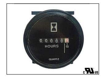
Provides precise tamper proof record of operating time of engines and other electromechanical devices. It mounts in standard 2" opening. Typical use is to monitor running time for vehicles and machinery for maintenance scheduling, warranty, rental use and service records. Locking snap-on retainer secures meter firmly to panel from the back. No visible fasteners.
