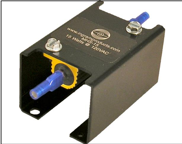
The mini space heater is designed for interior enclosures where space is at a minimum, and a limited amount of heat is required. Use it to keep the temperature inside an enclosure several degrees above the external ambient temperature and above the dew point. Keep your electrical equipment on line by preventing corrosion due to condensation. Contact our engineering department for specifications for the proper AHC or MHS model used in other types of enclosures (Aluminum, Fiberglass, etc.).
