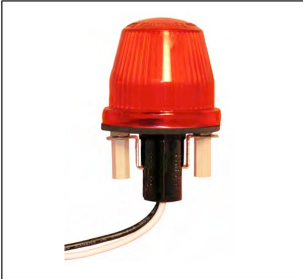
The Ingram LX10 is a NEMA and UL Type 3, 3R, 4, 4X, 12 and 13 low cost, low profile, panel mount alarm light suitable for heavy duty applications inside and outdoors. The lens is molded from shatter resistant GE Lexan. This alarm light is particularly useful on small panels.
