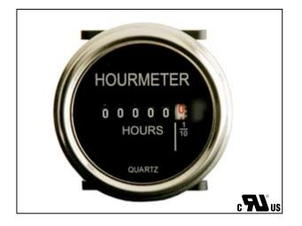
Provides precise tamper proof record of operating time of engines and other electromechanical devices. It mounts in standard 2" opening or 1.5" knock out. Typical use is to monitor running time for vehicles and machinery for maintenance scheduling, warranty, rental use and service records. Locking snap-on retainer secures meter firmly to panel.
