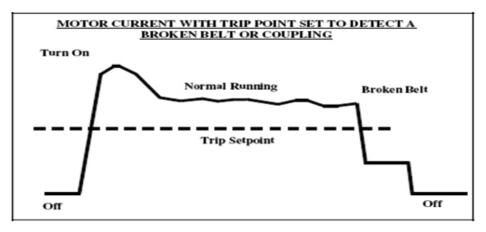
The output switch of all devices is normally open, when the monitored current exceeds the trip value as set by the multi-turn
