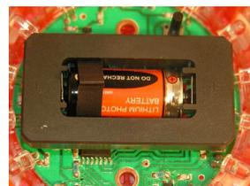
Replace battery. Ensure that the tabs are aligned when replacing the lid
