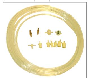
The Ingram bubbler kits are designed for Ingram TUF pumps to be used in bubbler type liquid level control applications. They must always be used in conjunction with the pump to prevent excessive back pressure and heat from developing that can shorten pump life. The BK-10 kit will maintain approximately 5 to 6 psi pressure for 0-10ft deep liquid reservoirs. The BK-20 will maintain 10 to11 psi for 0-20ft systems and the BK-30 will provide 14 to15 psi for 0-30ft systems.
