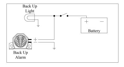
Backup alarms should be installed on the rear of the vehicle in a location that will provide protection from weather, and minimize the possibility of damage in the event of a collision. Alarms should be mounted approximately 4 ft above the ground with the face of the alarm directed toward the rear of the vehicle.
