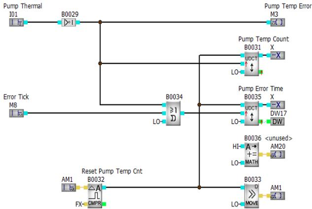
The circuit shown uses a time-on-delay triggered by the Pump Run signal going active. If the Contactor, such as a CHINT NC1 auxiliary contact closes within the programmed time the Contactor Error is held off. A counter is used to track the number of errors.
