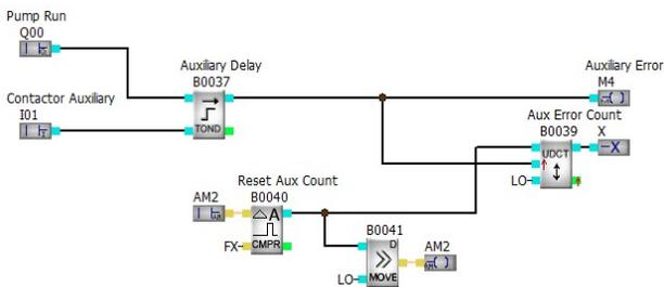
The circuit shown accepts a N/C input and if it opens it indicates that the Thermal Overload Relay has tripped which is treated as an Error condition.
