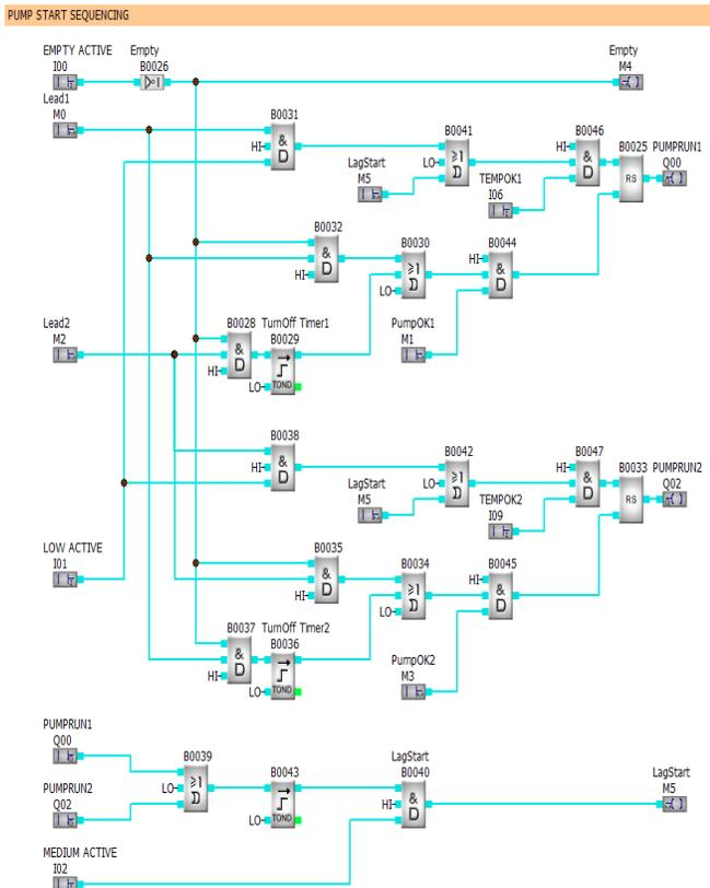
The pump start sequencer detects when the LOW signal is activated and will latch ON the current lead pump. If the MEDIUM input is activated the lag pump will latch on provided 8 seconds have elapsed from the lead pump turn on.
