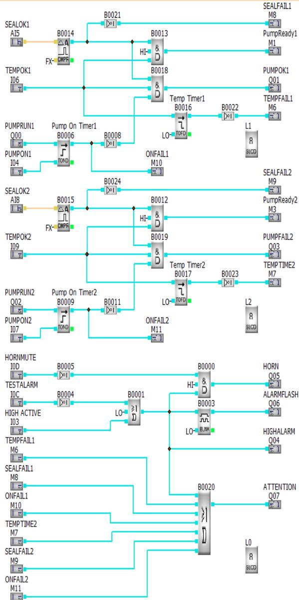
The PUMPONx signals are applied to a timer. If the pump has been activated a timer is started and if the PUMPONx signal is not applied within 4 seconds an error condition is reported.
