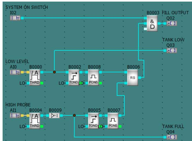
The output will control the filling of the tank by opening a valve or activating a pump. The outflow from the tank is not directly controlled, but a relay output will be provided to indicate when the tank level is below the LOW level.
