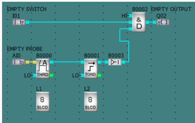
The only change required is the removal of the B0002 inverter. The probe signal now must be present to allow the empty process to proceed. Previously, the probe signal (FULL) had to be absent to allow the fill process to proceed.
