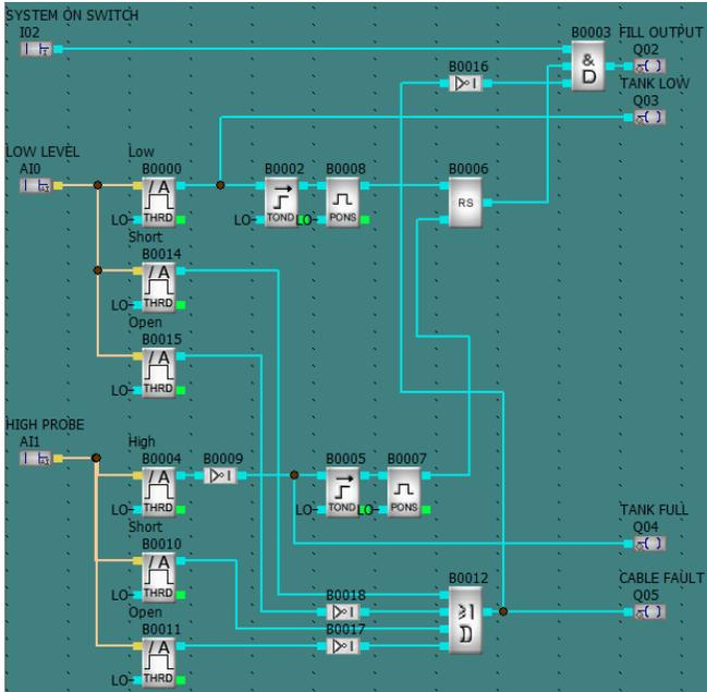
Threshold detectors B0010 and B0014 detect when the cable is shorted. Threshold detectors B0011 and B0015 detect when the cable is open. These signals are fed to an OR block B0012 that will activate the CABLE FAULT output if any inputs are out of the acceptable range.
