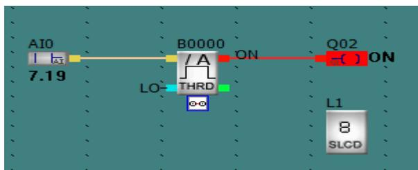
Double clicking the THRD block will display the associated parameters.
