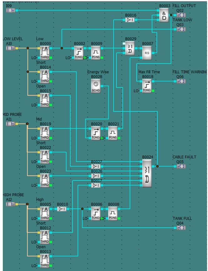
In operation, if the water level is below the LOW level sensor the FILL OUTPUT will be activated regardless of the time-of-day. If the MID level sensor is activated between 8:00 PM and 6:00 AM the FILL output will activate, allowing the pumps to operate using lower cost energy.
