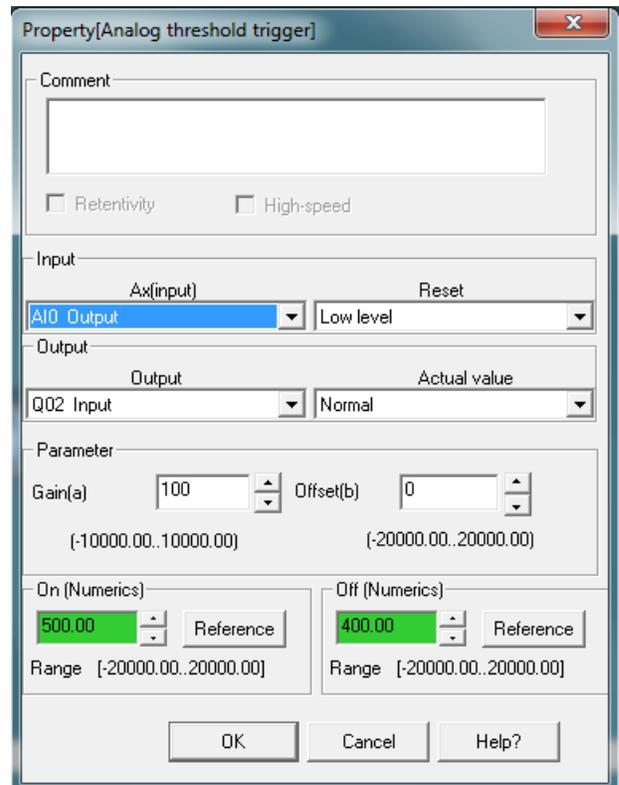
As shown, the 'On' threshold has been set to 500 and the 'Off' threshold has been set to 400.
