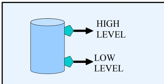
Once the tank starts filling it will continue until the HIGH level probe turns off the latch. The FILL output will not turn on again until the liquid has dropped below the LOW level probe.
