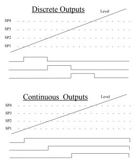
Two sets of outputs are provided, referred to as Level 1..6 and Alt Level 1..6 One set can be used to The output configuration option defines 3 different drive a pump sequencer and the second to drive indicators. Configuration options allow setting Level discrete.
