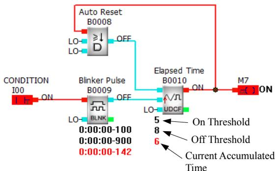
By replacing the simple Up/Down counter with an Up/Down Threshold Counter and adding an edge triggered OR gate the elapsed timer can be expanded to provide an output if the accumulated elapsed time exceeds a specific threshold and maintain the output until the accumulated elapsed time reaches a second threshold value.
