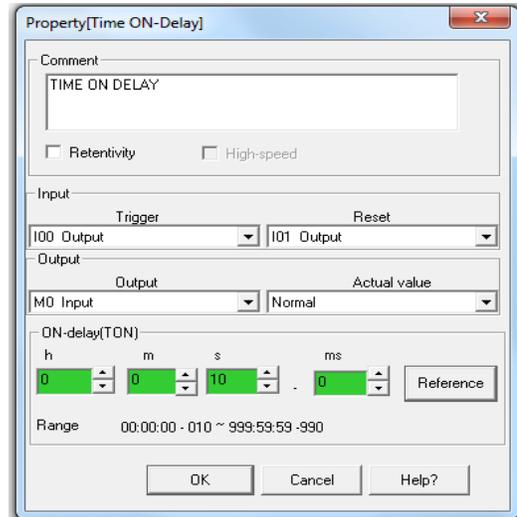
By selecting the 'Reference' option the preset may be tied to a Data Register DW0..DW255. Data registers may be directly set by the user from any of the 64 user defined display screens. Refer to AP-8 Run Time Monitoring for further examples.
