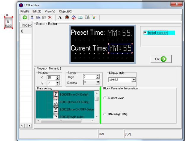
In the HMI configuration screen shown, the text 'Preset Time' and 'Current Time' can be any user defined text to describe the information. The **B** option allows displaying any block information, in this case block B0000 which is the Time ON delay shown in the first example. The MM:SS characters will be replaced with the actual timer values on the HMI display.
