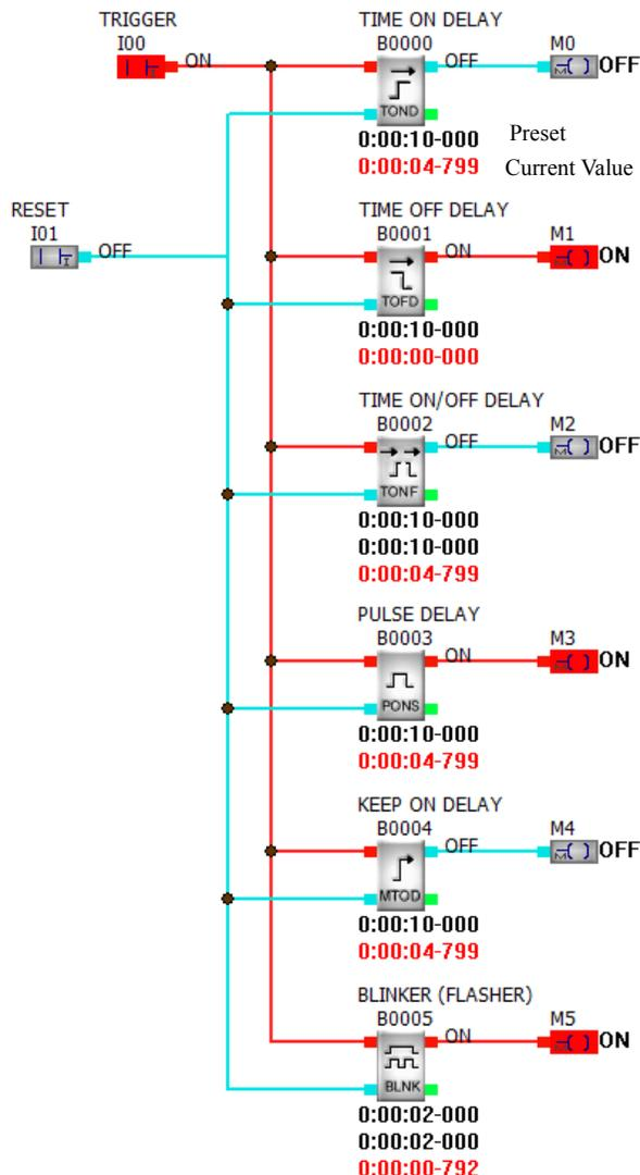
The integral timers all provide a timed output signal which is triggered from an input signal transitioning to a particular state. In all cases, when the input signal condition is removed the timer either resets or 'freezes' the output and when the input condition is re-applied the timer value is reset and the sequence repeats. There is no mechanism to 'stop' and 'restart' the timers.
