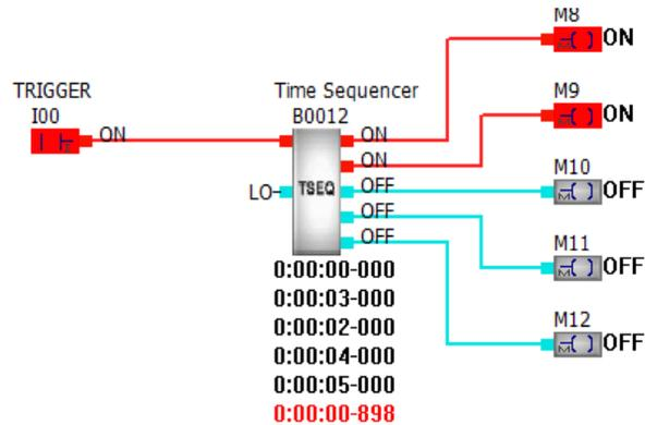
When the TRIGGER input is active the Step Sequencer timer is running. The Step Sequencer may be configured with up to 8 outputs (5 shown) and each output has a preset time. When the timer reaches the first preset the first output will become active and the timer resets to 0 and starts
