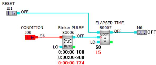
If the 'CONDITION' and 'RESET' inputs are configured to a permanent 'HI' level the Blinker will run whenever power is applied to the APB controller and the current value of the counter will show the total running time of the unit.
